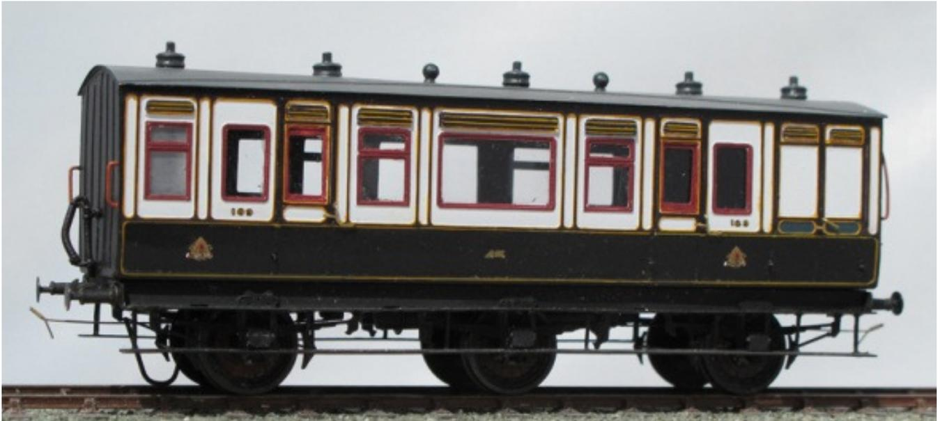
The LNWR had a large number of 6 wheel carriage types, in 30' 1" and 32' lengths. Initially the kits are for the later, shorter but more common versions. The kits feature a .012" etched brass body, a Cleminson truck underframe etched in .015" nickel silver and cast brass and whitemetal detailing parts. The roofs are vacuum formed plastic and screws, wire, etc are also included. 3' 6" Mansell pinpoint axle wheels, with waisted pin point are required to complete the model.
