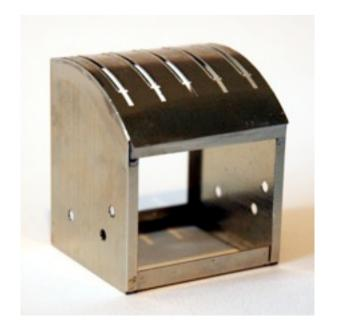
Solder the frame side plates and bars 3&4 together ensuring that the frame is square in all directions. The lower bars (3) fit inside the bottom and side folds, the top bars (4) (without the rodding guide holes) attach outside the side folds.
