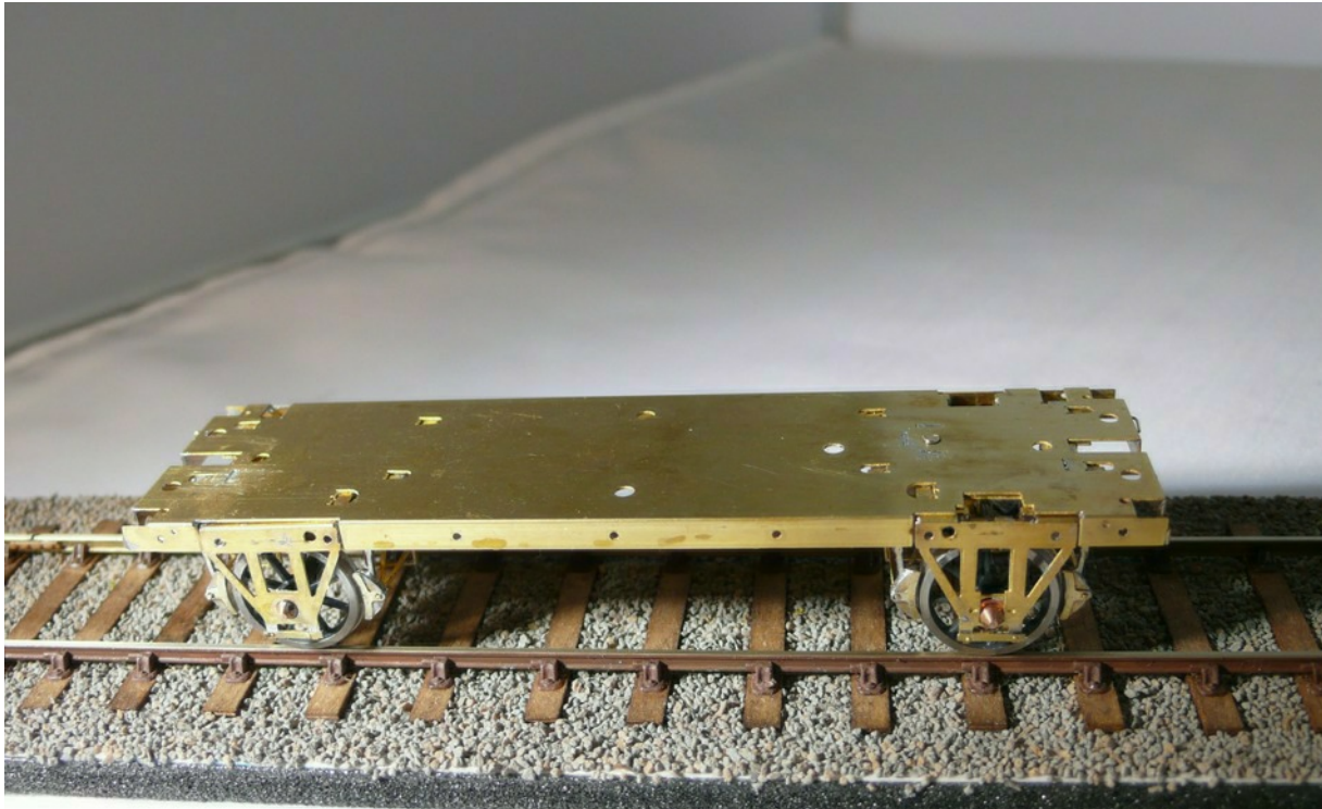
AA13 20T Toad clasp braked underframe showing the adjustable W-iron side. The conspicuous sand pipes are yet to be fitted. A bending jig and setting etch is planned to simplify making the sand pipes and fitting them.
