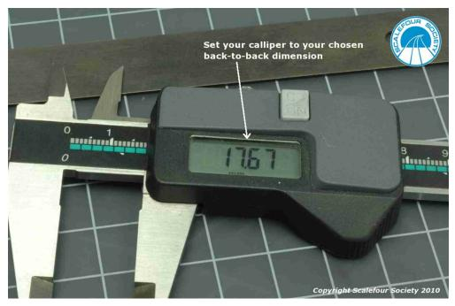
The next step is to align the calliper blades on the straight line on your flat surface. You should insert the small end of the Gauge between the calliper jaws and slowly pull it along between them until it comes to a natural stop. Do not try and force it through the gap as you do not want it to become wedged between the jaws.
