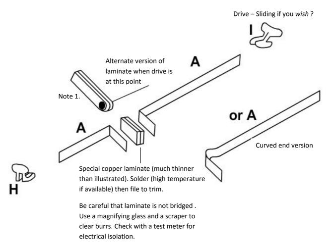
Note 1. If laminate is used in extended form, ensure that driving rod does not short two sides of laminate by clearing the hole on one side and only soldered on the other.
