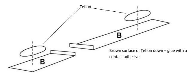
The base plate is to be glued onto an un-riveted wide sleeper. Teflon pads as shown. Do not allow the two sections of **B** to touch in order to avoid the possibility of shorting although the Teflon does help.
