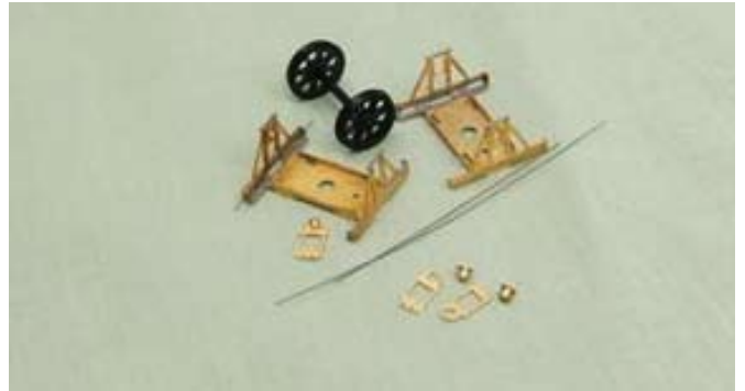
Springing, where the suspension mimics the full-size wagon, is a newer development but, having said that, the author has two sprung wagons which are 14 years old. Illustrated is a pair of sprung units to Bill Bedford's design plus a wheelset of open spoked wheels. Here both units are fixed to the wagon but the wheels, with pin-point axles, run in bearings which are allowed to move up and down in the suspension units controlled by spring steel wire. The components for one four-wheeled wagon are shown (less one wheelset) with a bearing, spring carrier and spring in position on one unit. Don Rowland
