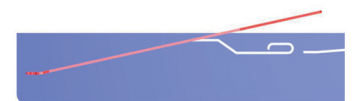
STAGE 66 First bend of Morton lever. Note cam positioned upwards, complete as for standard lever.
