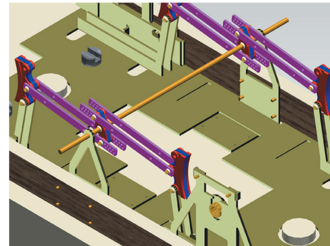
STAGE 101 FIXING 3: Fitting brake levers for MORTON brakes. Discard red V hangers, fit wires and repeat other side.
